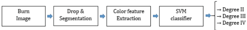
Fig. 5. SVM classifier applies for burn image. This figure shows diagram of SVM burn image classification from the burn image input to the degrees of burn output.
