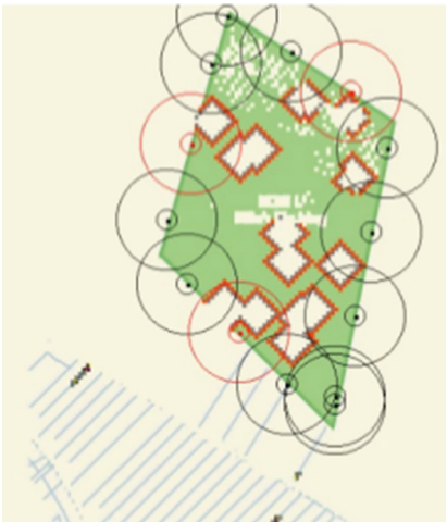
Fig. 10. The interoperability of four federates under the context of the mixed simulation: river, forest, WSN, and observer. The sensors changed to red color since the fire was detected close to them (Color figure online).
