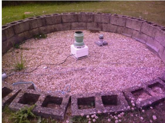
**Fig. 2.** The disdrometer and a co-located rain gauge at Chilbolton Observatory.
