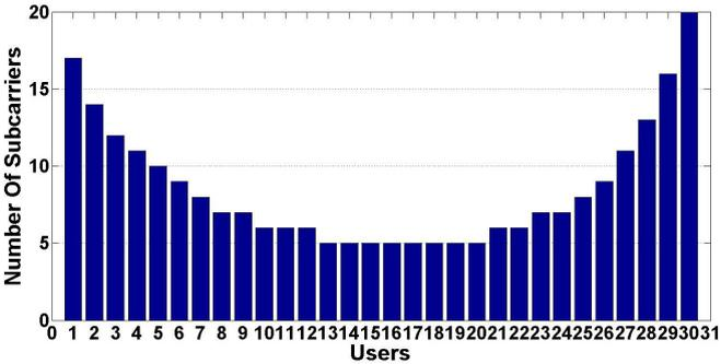
**Fig. 5.** Subcarriers allocation for smaller range of increasing discount factor:  $\delta_{i+1} = \delta_i + 0.003$ ,  $\delta_1 = 0.893$ .
