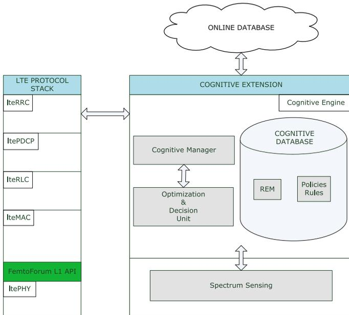
Fig. 3. SW Architecture of the Cognitive Extension
