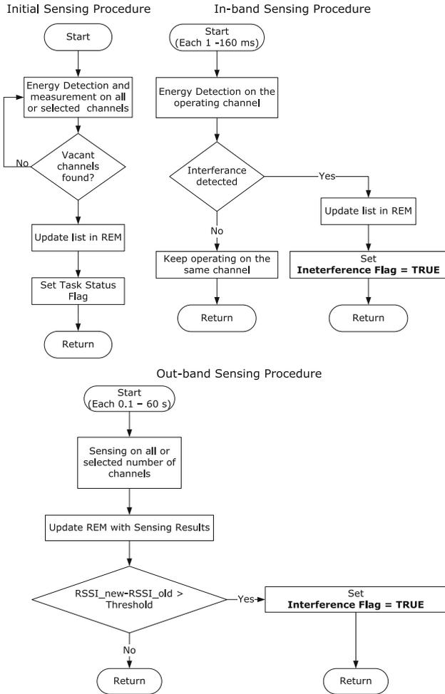
Fig. 2. Sensing Procedures
