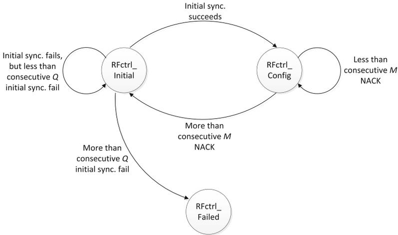
**Fig. 6.** Finite state machine in the master node
