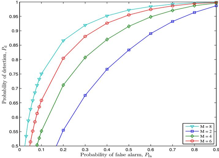
**Fig. 1.** The complementary ROC of the proposed GLRT-based detector for  $SNR = -8$ ,  $P_{fa} = 0.01$ ,  $N = 32$ ,  $L = 10$  and different value of  $M$ .
