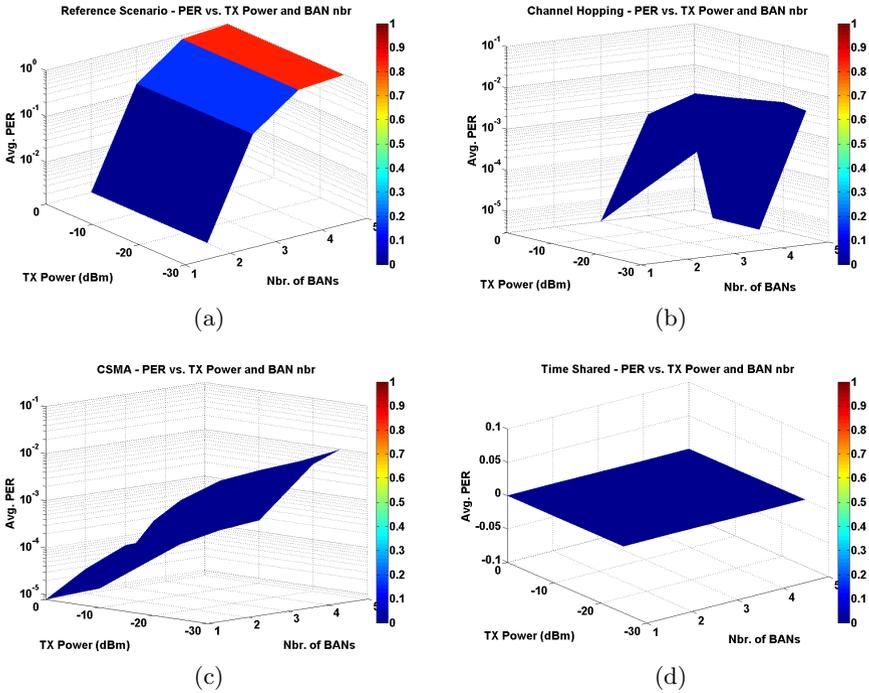
Fig. 3. Packet Error Ratio Distribution of Coexistence Schemes, (a): Reference Scenario, (b): Channel Hopping, (c): CSMA/CA and (d): Time shared
