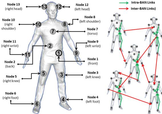
**Fig. 1.** Intra-BAN and Inter-BAN Networks and Interference Scenarios.
