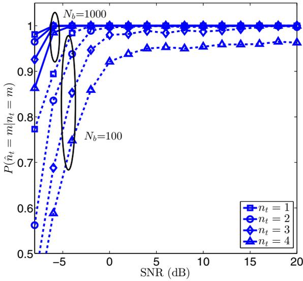
**Fig. 1.** The probability of correct detection,  $P(\hat{n}_t = m | n_t = m)$  versus SNR for different  $n_t$  and  $N_b$  values.
