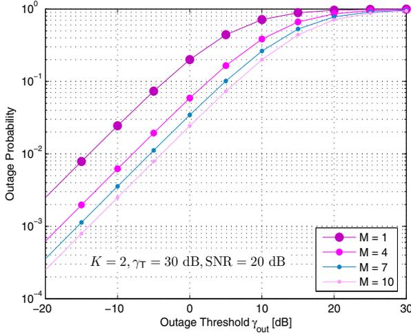
**Fig. 3.**  $P_{out}$  vs  $\gamma_{out}$  for different values of  $M$  and  $\mu_{s,m} = 20$  for  $m = 1, \dots, M$ ,  $\Omega_{s,r} = 0.8$ ,  $\mu_{r,m} = 0.01$  for  $m = 1, \dots, M$ , and  $\Omega_{r,k} = 0.9$  for  $k = 1, 2$ .
