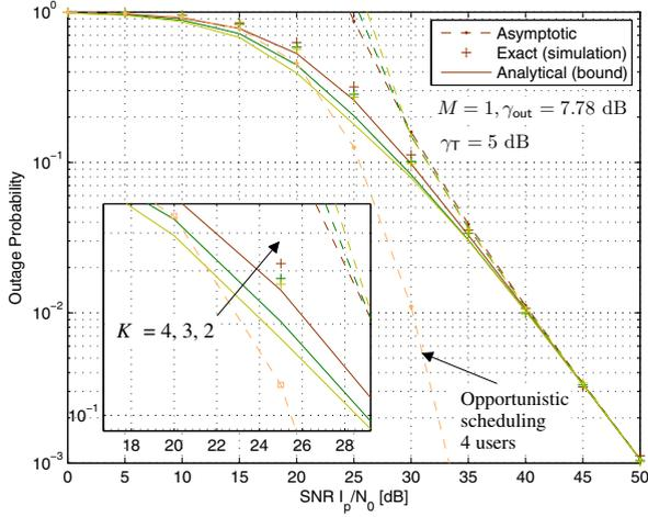
**Fig. 2.**  $P_{out}$  vs SNR for different values of  $K$  and  $\mu_{s,p} = 30$ ,  $\Omega_{s,r} = 0.8$ ,  $\Omega_{r,p} = 0.1$ , and  $\Omega_{r,k} = 0.7$  for  $k = 1, \dots, 4$ .
