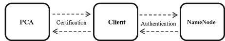
Fig. 5. The high level processes of our TPM-based Hadoop authentication protocol (Client to NameNode in this example).
