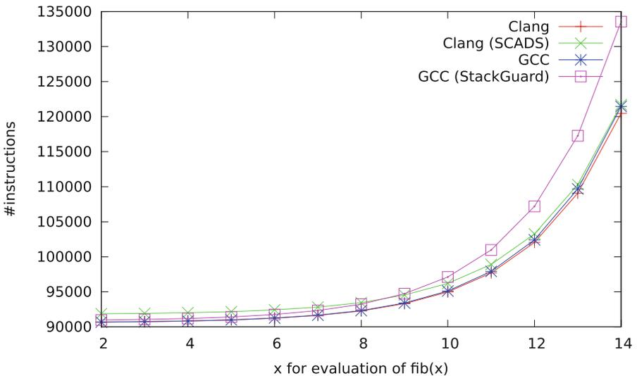
**Fig. 3.** Number of instructions for the recursive computation of a Fibonacci number.
