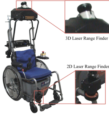
Fig. 1. Our developed autonomous wheelchair.
