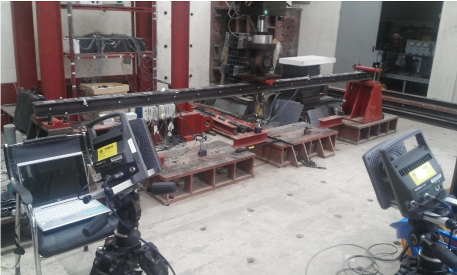
Fig. 2. The Installation View of The Steel Beam Experiment
