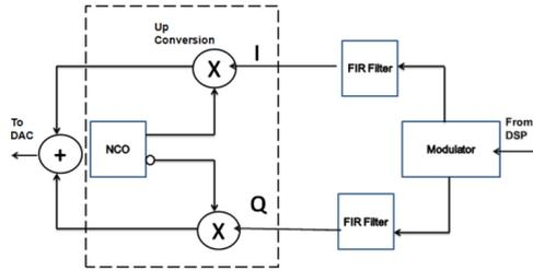
Fig. 2. Digital Frontend Transmitter
