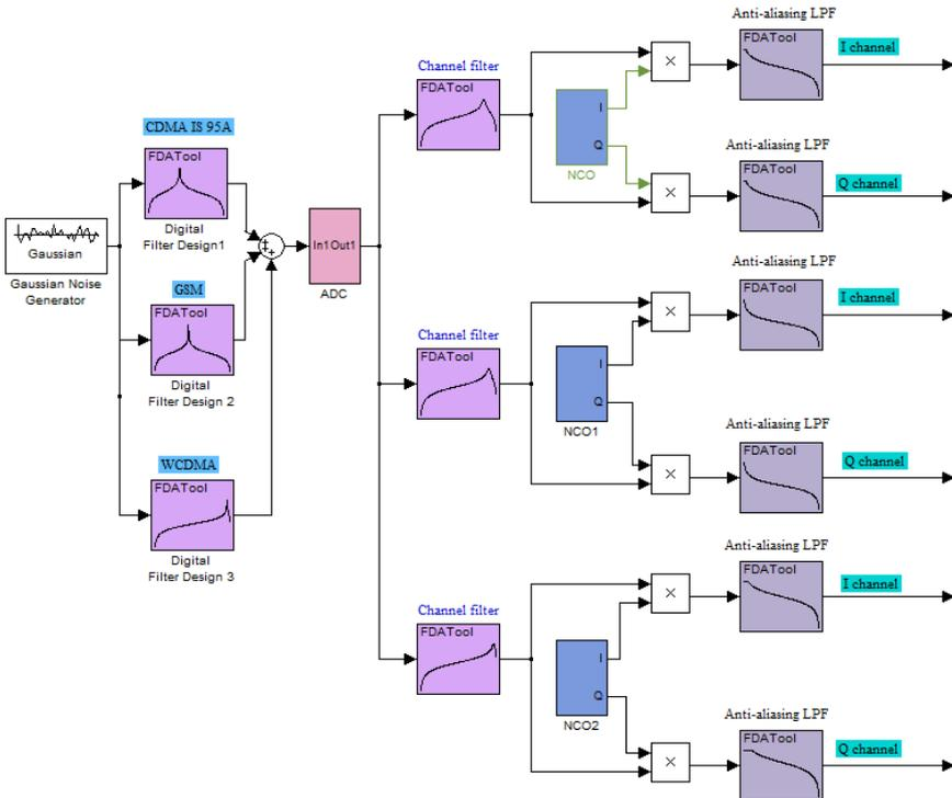
Fig. 3. Software based RF Frontend Receiver
