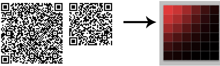
Fig. 4. Two QR codes that carries the pixel values of a 6 by 6 pixel image
