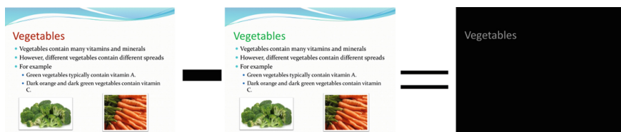
Fig. 6. Finding the bounding box by diffing two images.
