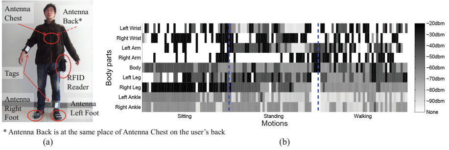
Fig. 3. (a) Wearable RFID system, (b) average RSS readings with different motions over time.
