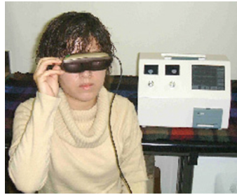
Fig. 5. The improved measuring unit with gaugle
