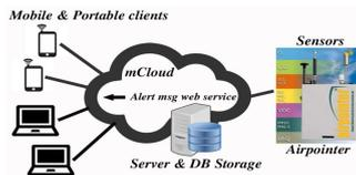
**Fig. 1.** Architecture of the Air Quality Monitoring System
