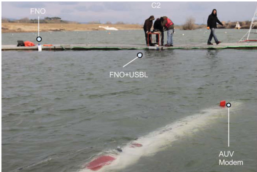
Fig. 7. Area of experimentation during one of the test on February 7. The AUV is visible in the foreground, while the two fixed nodes are deployed in the water close to the pier, as signaled by a white buoy on the left (FNO) and by a grey box connected to the C2 (USBL).
