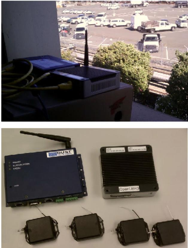
**Fig. 9.** Long-term deployment setup at the Chevron-Richmond refinery. The result of this test was a detection rate of 100% with no false alarms. The sensors withstood strong winds and rainy weather.
