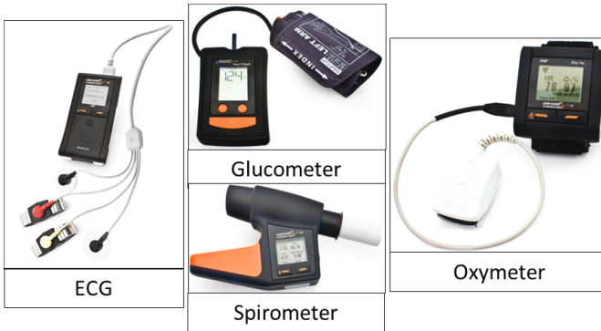
Fig. 6. Vidavo eHealth Devices. Different vital signs with different clinical value are observed. Captured data is sent over Bluetooth to the application.
