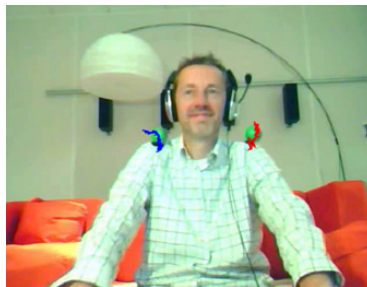
Fig. 3. Two green spheres placed on the user's shoulders are tracked in real-time (red and blue trajectories)
