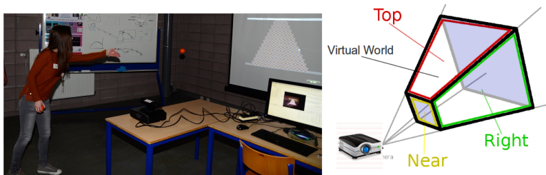
Fig. 1. Left: Live demonstration of the KinectBalls prototype. Right: The projection matrix (frustum) of the 3D virtual world.
