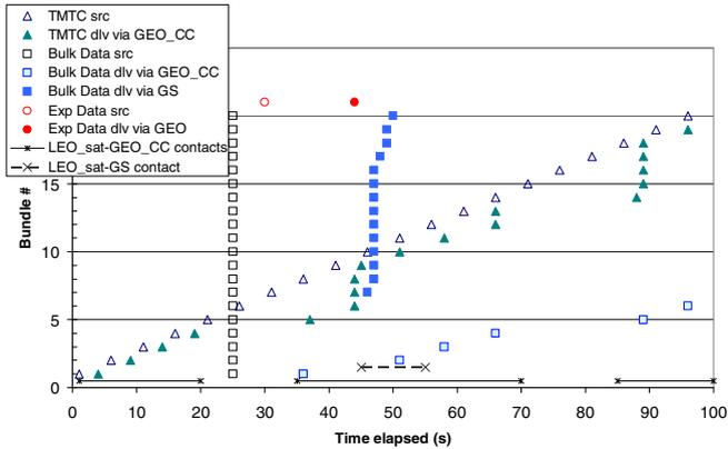
**Fig. 7.** Overall bundle traffic. Bundle telemetry (from LEO\_sat to LEO\_CC, always via GEO\_CC) and Bundle data (from LEO\_sat to User, either via GEO\_CC or GS).
