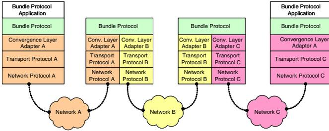
Fig. 1. DTN Bundle Protocol architecture and protocol stack
