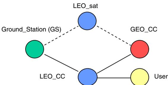
**Fig. 2.** Topology of the LEO-GEO scenario. Dotted lines: intermittent sat links (LTP); continuous lines: continuous terrestrial links (TCP).
