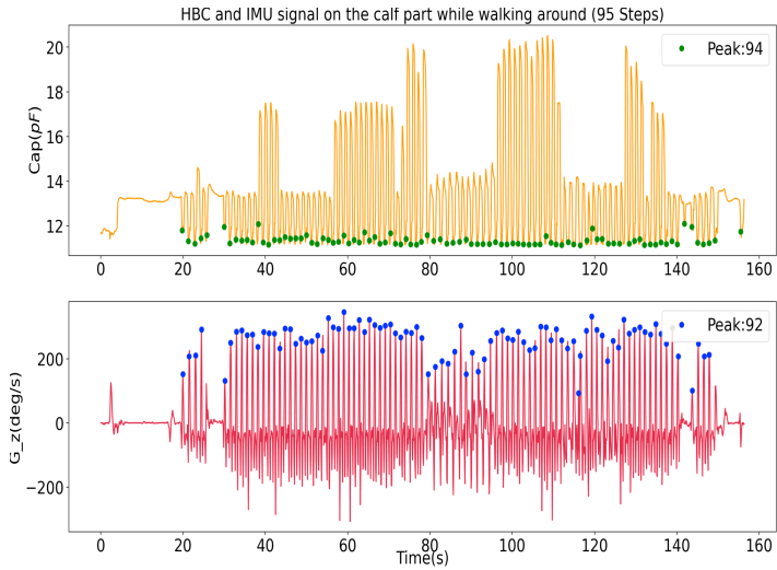
Fig. 15. Peak detection for step counting
