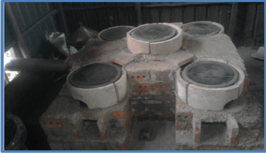
Fig. 4. Improved institutional mirt stove prototype
