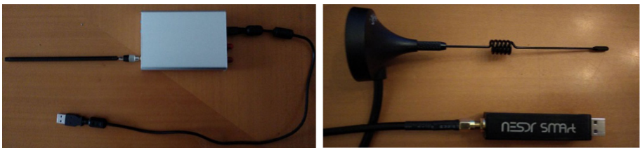
Fig. 6. SDR transmitter setup (left) and SDR capture setup (right).
