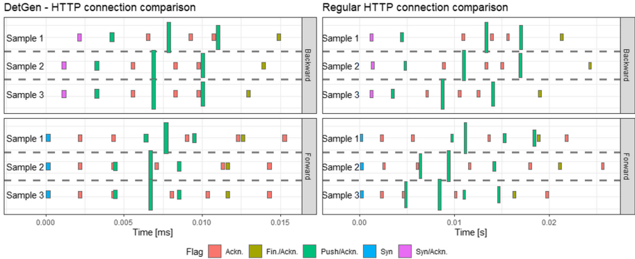
Fig. 7. Packet-sequence similarity comparison for HTTP-activity for DetGen and a regular setting.
