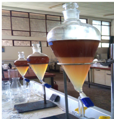
Fig. 5. Washing biodiesel (soap is at bottom)
