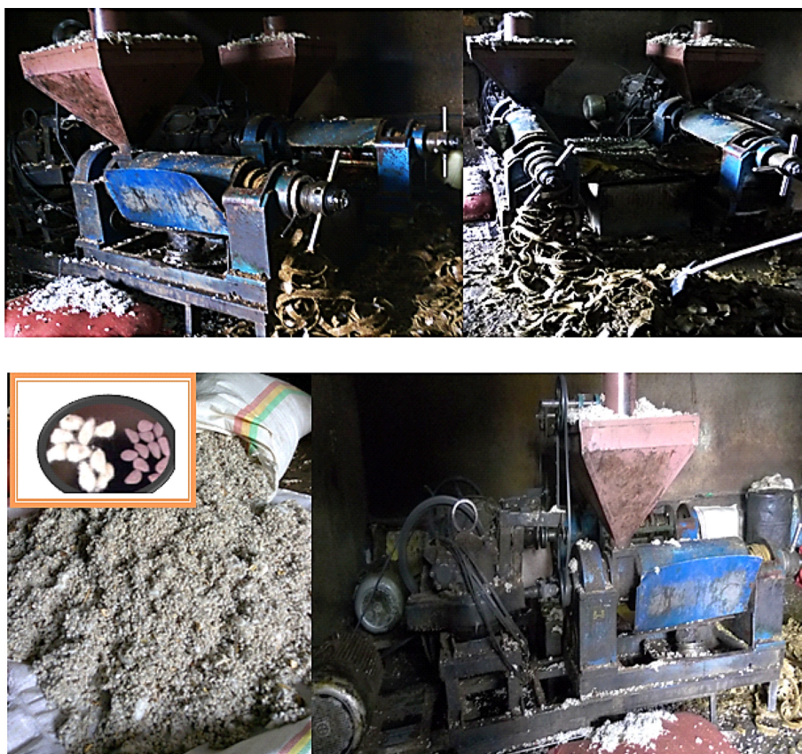
Fig. 1. Extraction of oil from cotton seed by screw pressing.
