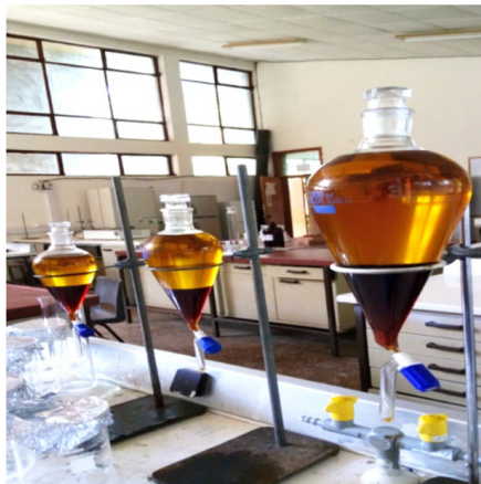
Fig. 4. Glycerol Separation from methyl ester
