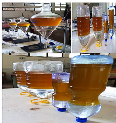
Fig. 6. Final washing of biodiesel
