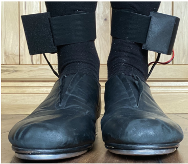
(a) Front view: Power switch and cable holes face backwards
