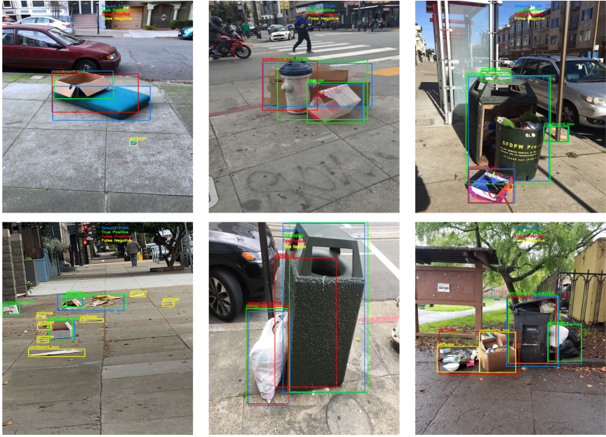
Fig. 13. Object detected images with some error generated from RetinaNet (Color figure online)
