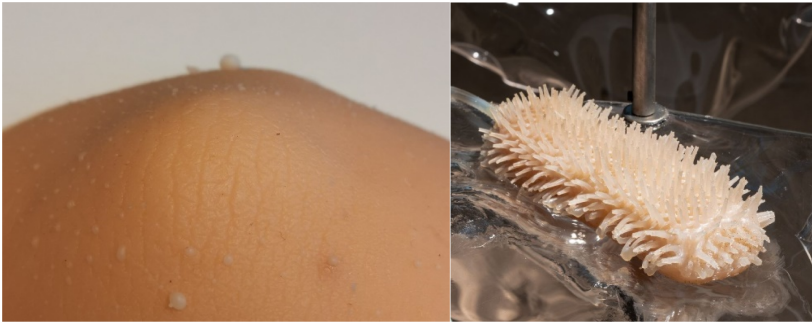
Fig. 7. Skin texture cast in silicone using a mold made from alginate by depressing an elbow into it (left). Small tentacles cast in silicone onto a soft robotic actuator using a mold made from clay (right). Right image courtesy of Studio ThinkingHand, detail from their work INTERTIDAL SYNTHESIS (2020), 3 channel video and sculpture installation.
