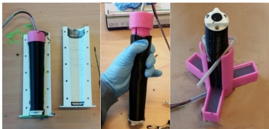
Fig. 5. Demolding and bonding of the two tentacle parts
