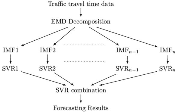
**Fig. 7.** Process schema of EMD-SVR method.
