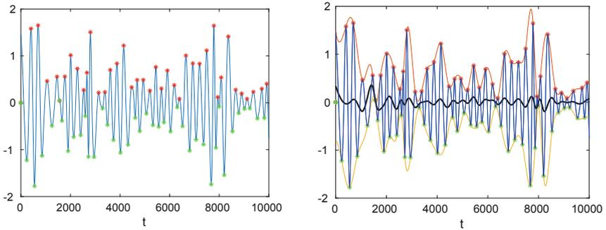
(a) All local maxima (red points), and local minima (green points). (b) Construction of the mean curve by applying a cubic spline.
