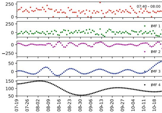
**Fig. 6.** The original data for the average travel time for the window 07:40–8:00 and the intrinsic mode functions (IMFs) by applying empirical mode decomposition (EMD). The upper signal is the original data, and the subsequent four signals are the IMFs obtained by applying EMD to the original data.
