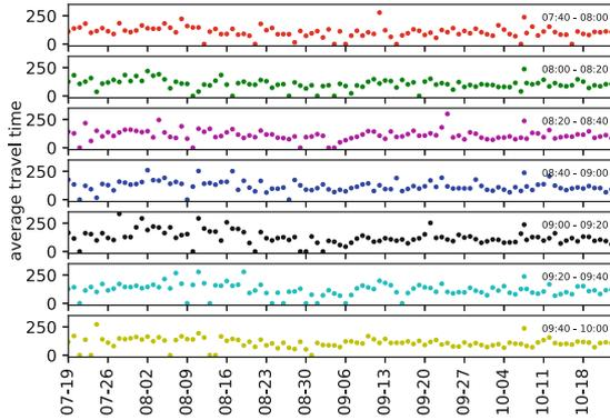
**Fig. 5.** The rush-hour average travel time data for the route B-3 for the dates 19-07-2016 to 24-10-2016. The data for the time-window 07:40–8:00 are also added since they were used to predict the first rush-hour window, 08:00–8:20.
