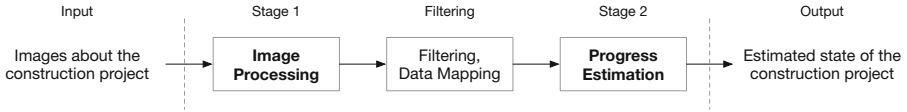
Fig. 2. Overview of the estimation pipeline. The two major parts of the system are an image processing network (e.g., for semantic segmentation) and a stage classification to predict the project’s state.
