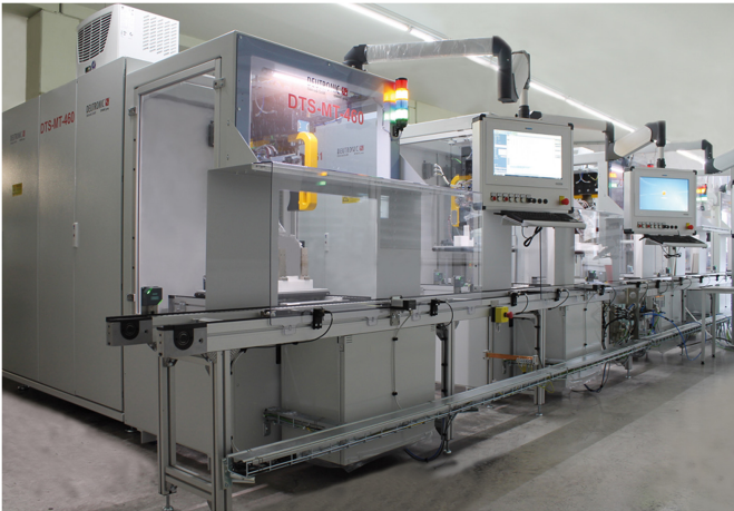
Fig. 3. Example of a real EOL test system station. EOL MT460 Motortester [18].
