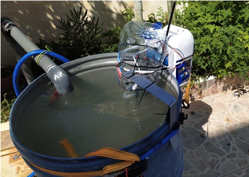
Fig. 4. Sensor node in a plastic drum with real river water sample.
