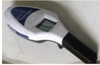
Fig. 1. Device used to gather data from NDVI of each plot.
