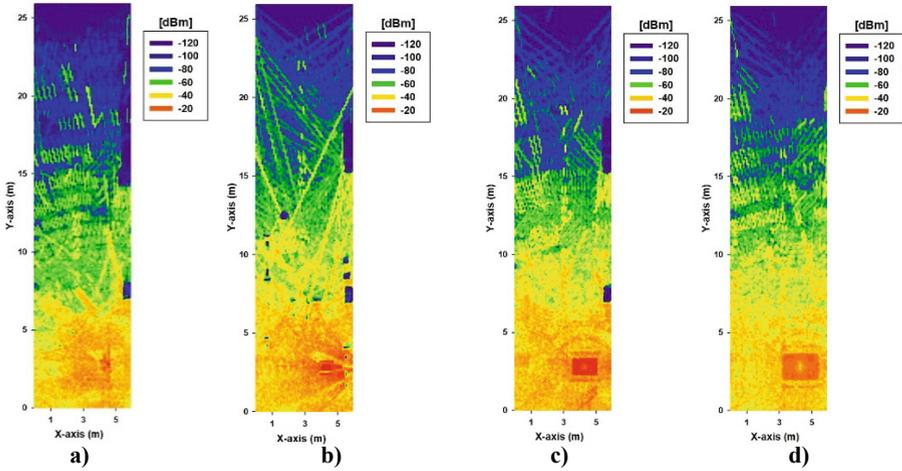
**Fig. 4.** Received power levels estimations for the SUT, corresponding to a frequency of operation of 2.4 GHz, and cut-plane heights of a) 0.6 m, b) 1.2 m, c) 1.8 m and d) 2.4 m respectively
