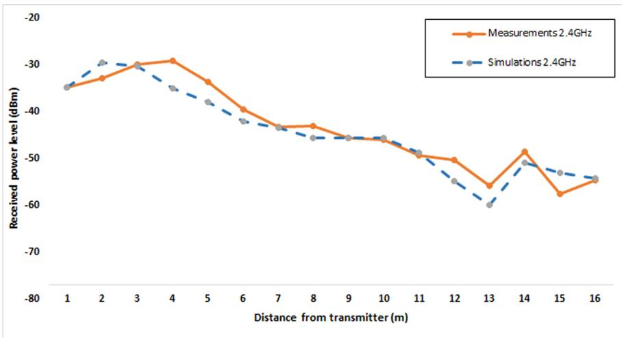
Fig. 9. Comparison of simulation vs measurement results for the Scenario Under Test, considering transceivers operating at a frequency of @2.4 GHz.
