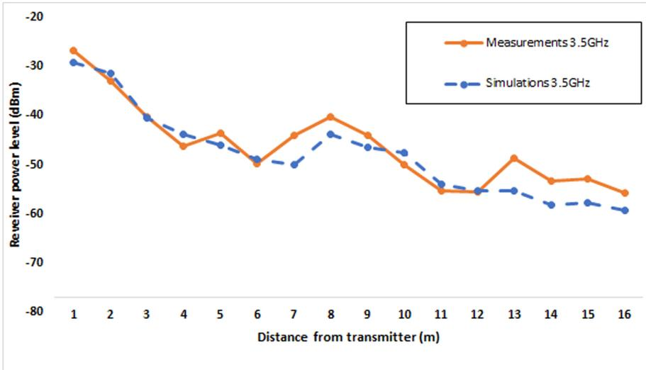
**Fig. 10.** Comparison of simulation vs measurement results for the Scenario Under Test, considering transceivers operating at a frequency of @3.5 GHz.
