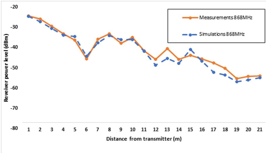
Fig. 8. Comparison of simulation vs measurement results for the Scenario Under Test, considering transceivers operating at a frequency of @868 MHz.
