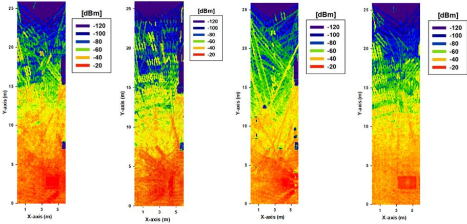
**Fig. 2.** Received power levels estimations for the SUT, corresponding to a frequency of operation of 433 MHz, and cut-plane heights of a) 0.6 m, b) 1.2 m, c) 1.8 m and d) 2.4 m respectively.
