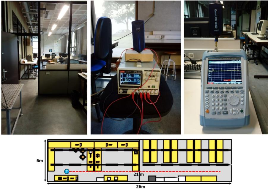
**Fig. 6.** Measurement scenario and schematic description of the measurement points within the Scenario Under Test, located at the Luis Mercader laboratory, at the Public University of Navarra.
