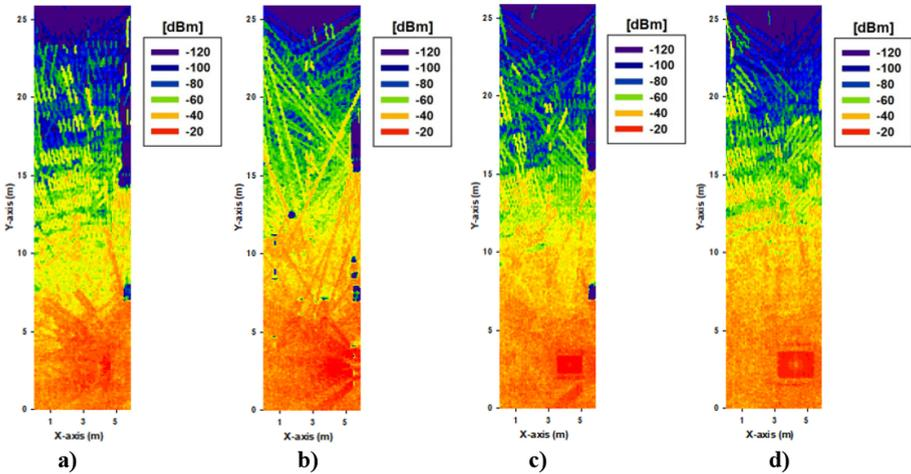
**Fig. 3.** Received power levels estimations for the SUT, corresponding to a frequency of operation of 868 MHz, and cut-plane heights of a) 0.6 m, b) 1.2 m, c) 1.8 m and d) 2.4 m respectively.
