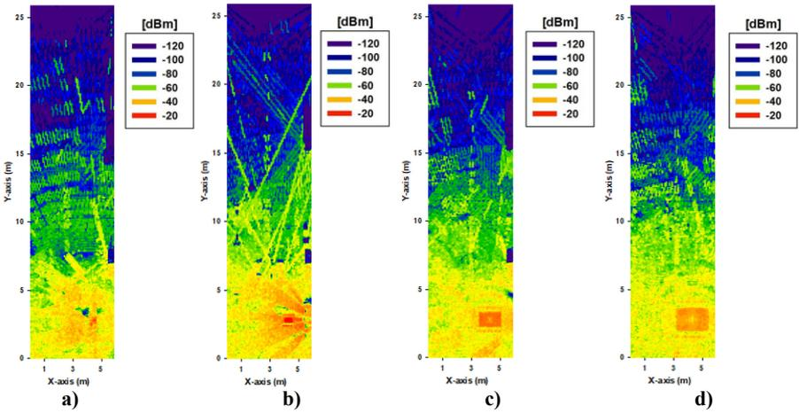
**Fig. 5.** Estimation of received power levels for the SUT, corresponding to a frequency of operation of 3.5 GHz, and cut-plane heights of a) 0.6 m, b) 1.2 m, c) 1.8 m and d) 2.4 m respectively
