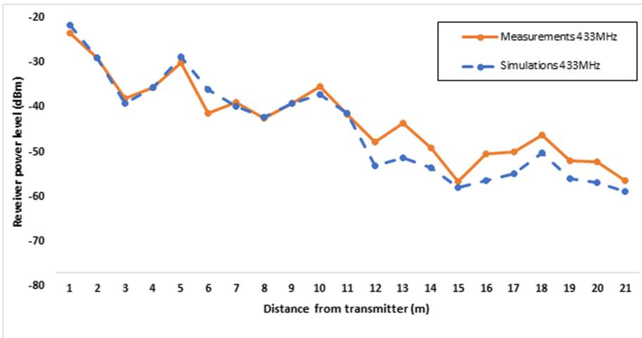
**Fig. 7.** Comparison of simulation vs measurement results for the Scenario Under Test, considering transceivers operating at a frequency of @433 MHz.
