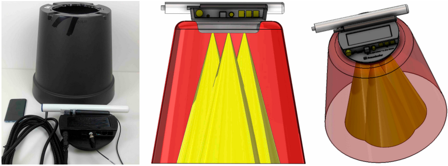
Fig. 5. Prototype and validation of the cabinet for controlled light.
