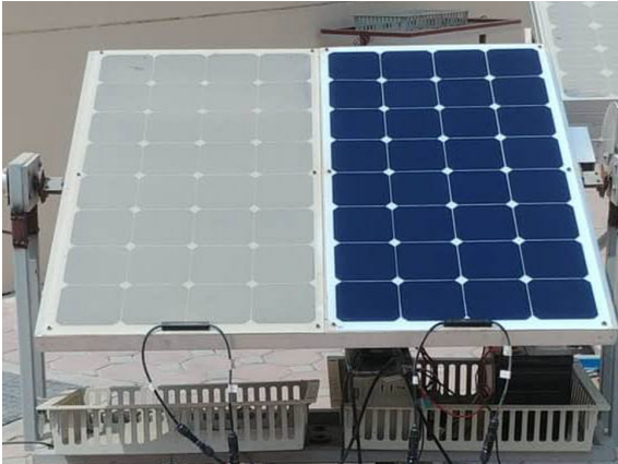
Fig. 2. The dusty and clean solar panels at the end of the testing period
