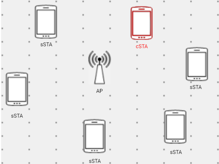
Fig. 2. Schematic diagram of network topology
