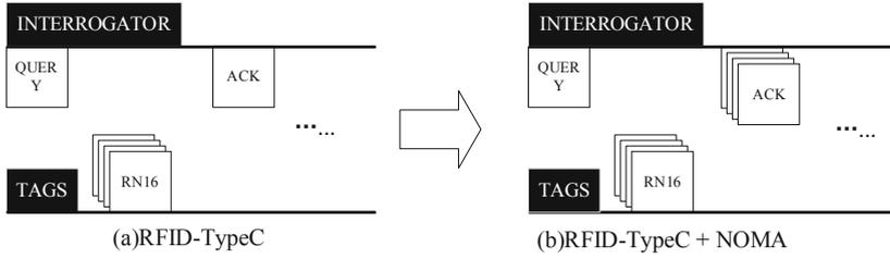
Fig. 6. Design of RFID-Type C identification frame based on NOMA.
