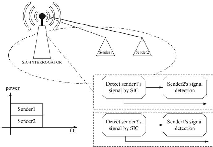
**Fig. 2.** Power domain NOMA Uplink Principle.
