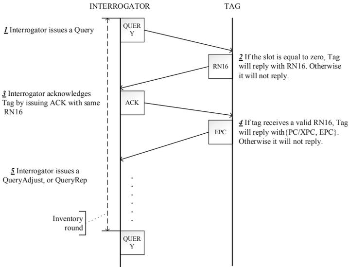
Fig. 1. Steps of an Interrogator inventories and access of a single Tag.
