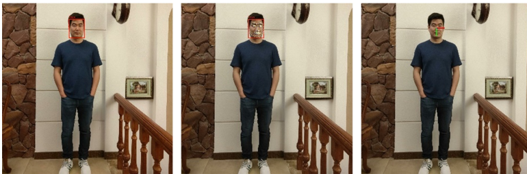
Fig. 5. (a) SSD face detection effect (b) Face feature point extraction effect (c) Head pose estimation result
