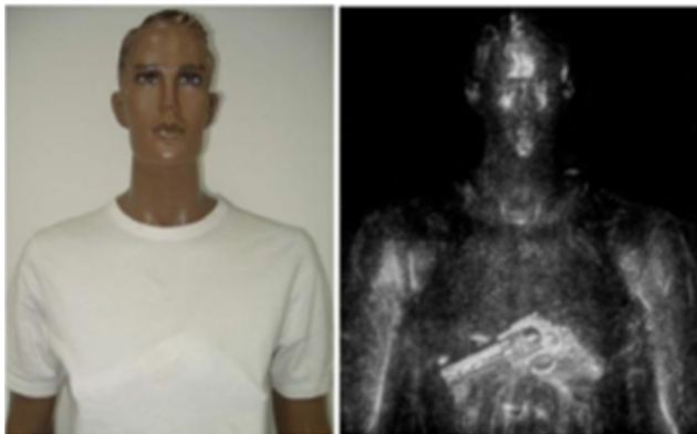
Fig. 5. 3D imaging results of a human model with a hidden pistol
