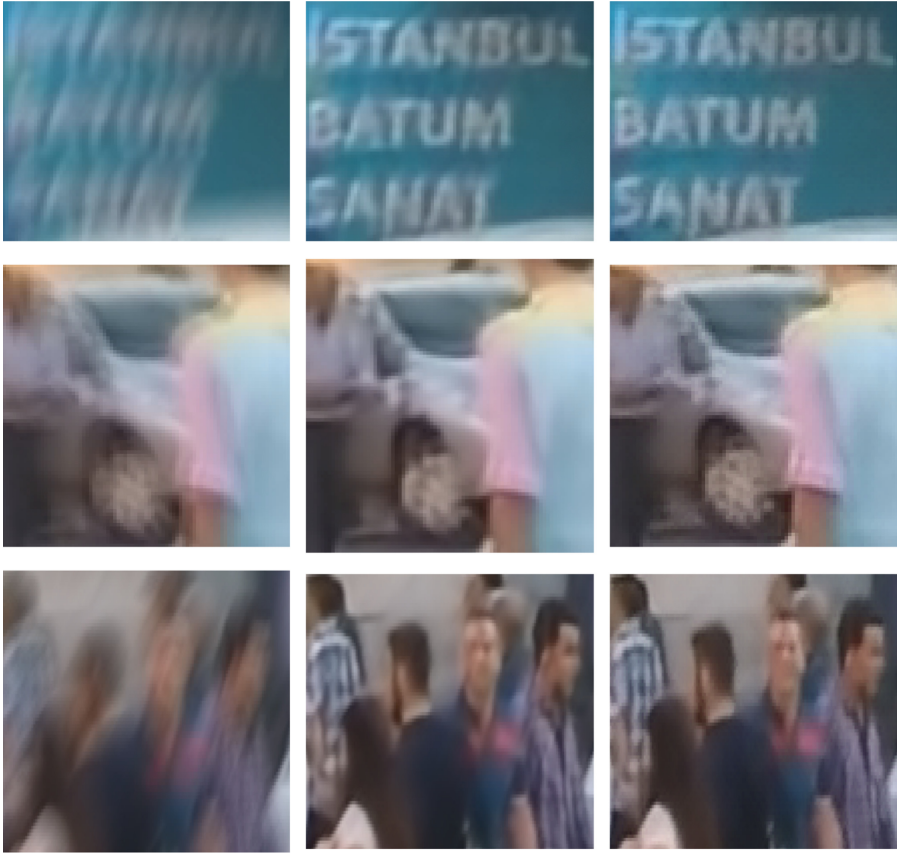
Fig. 5. Visualization of image quality enhancement with different losses. The first column is the original blurred image. The second column is the result with MSE loss. The third column is the result with MSE loss and perceptual loss.
