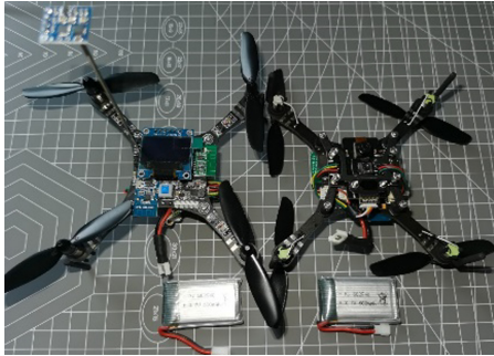
Fig. 5. Self-developed four-rotor UAV test platform
