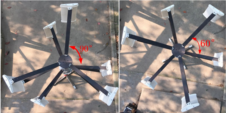
Fig. 13. Wind turbines at 90° and 60° double-layer installation angle
