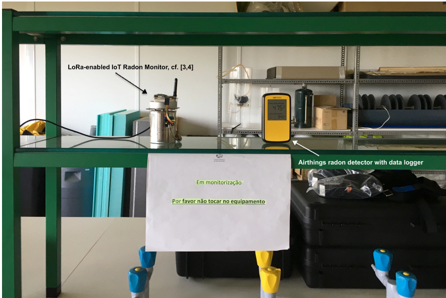
Fig. 4. The placement of the radon detectors in the Lab.
