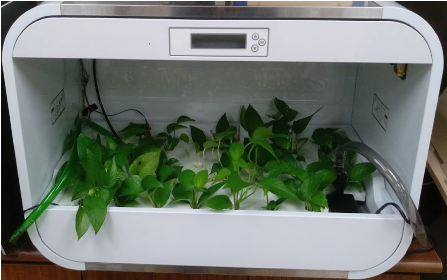
Fig. 1. The hydroponic plant box
